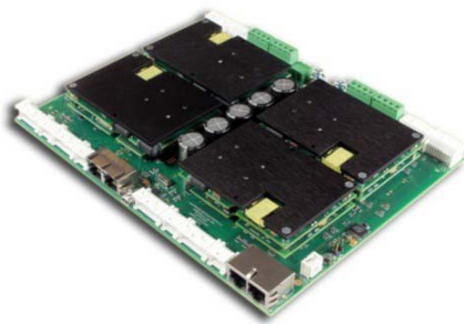
Figure 7 – Four plug-in servo drives mounted to create a 4-axis servo drive module
