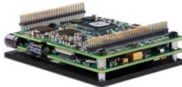
Figure 5 – DZE, EtherCAT plug-in servo drive (slave node)
