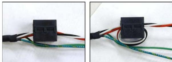
One turn is shown on the left and two turns on the right. Notice that the ground and shield wires do not pass through the ferrite.
