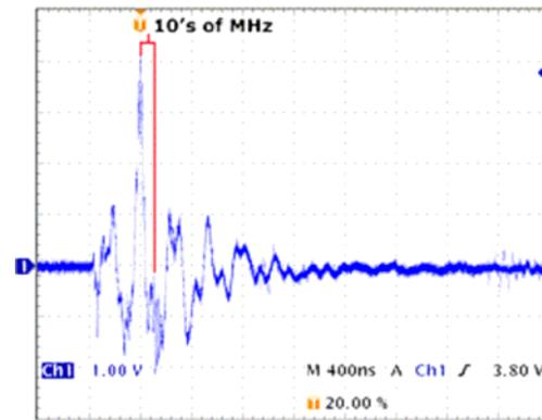
The drive is switching at 20kHz but the noise spikes occur at twice the switching frequency. Zoomed in on a single spike it is apparent that the frequency is in the Mega Hertz (typically 5-50MHz).
