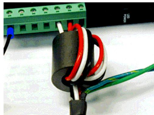
This ferrite has been placed as close to the drive as possible. Again, the ground and shield wires do not pass through the ferrite. This image shows three turns.
